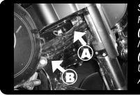
Stock Harness and Amplifiers Harnesses Passing from Fairing to Just in Front of Tank (Arrow A). Cable Tying the Harnesses To The Main Bike Harness Just In Front Of The Tank (Arrow B) Allows The Amp Harnesses To Go Up Towards The Tanks Chrome Console Easier And Makes For a Cleaner Install.
