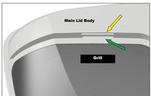
The yellow arrow shows a 2" long "slot" in the lid body where a 1-7/8" tab on the grill (shown by green arrow) slides into, further securing the grill to the lid. The grill cannot mount to the lid unless this tab is correctly seated.
