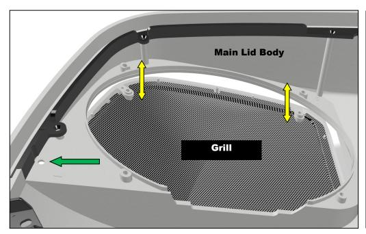
The yellow arrows are where speaker mounting screws go through the lid, through the speaker mounting holes and into the "bosses" on the grills to properly secure the grills.
